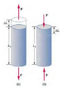
Compressive stress is the opposite of tensile stress. Instead of being stretched, the material is being compressed. The rod shown to the right in the figure above is experiencing compressive stress. Columns that support great weight are examples of members being subject to great stresses. The same mathematical relationship is valid for both tensile stresses and compressive stresses.
